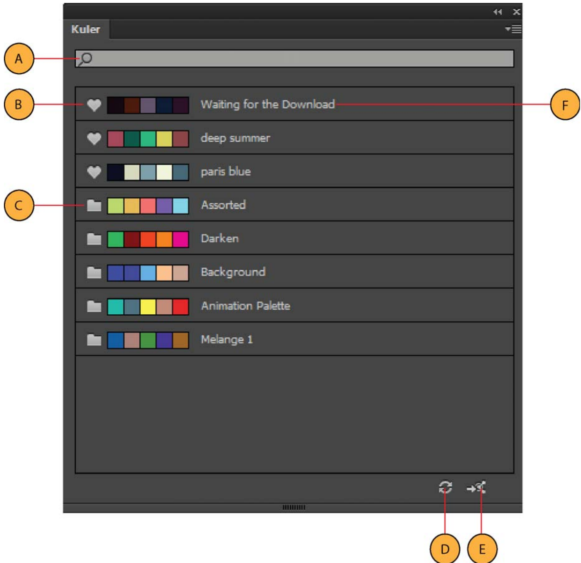
A Theme search by name B Favorite theme icon C Theme folder icon D Refresh E Launch Color website F Theme name
