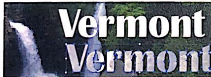
Flattening creates raster images with the pixels altered to create the same apparent effect as the semi-transparent text. The vector outlines of the original type mask the new raster elements.
