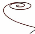
Figure 5-46 The helix spline with three turns and +1 value in the Bias spinner
