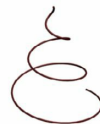
Figure 5-45 The helix spline with three turns and zero value in the Bias spinner
