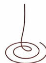
Figure 5-47 The helix spline with three turns and -1 value in the Bias spinner
